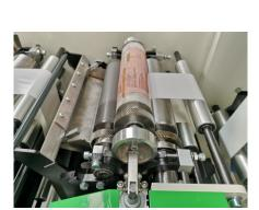
Flexographic printing unit with the quick lock system.
