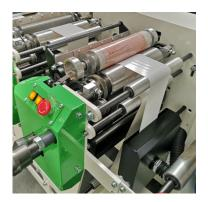
Modularity in design. Additional flexographic printing units can be added transforming it into a real industrial grade 6 color label printer.
